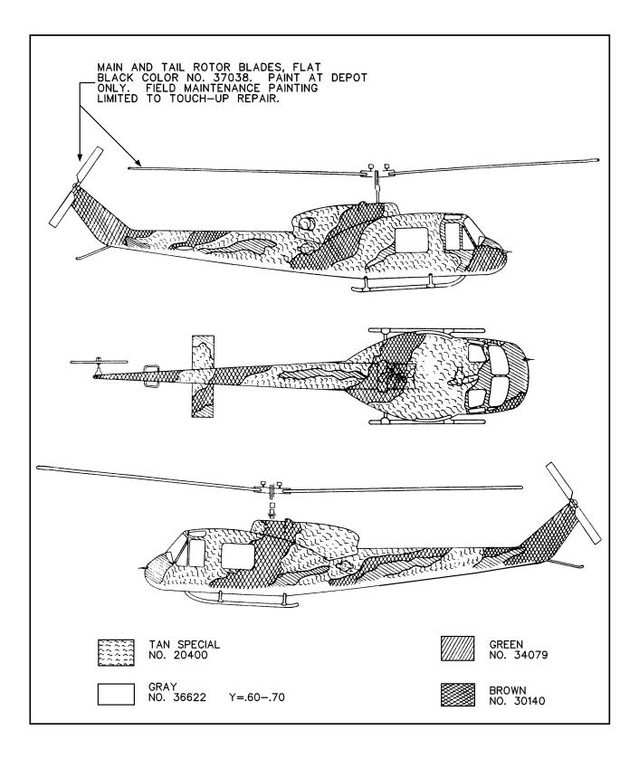
Figure D-18. UH-1F/D/N/H Aircraft Camouflage Pattern
