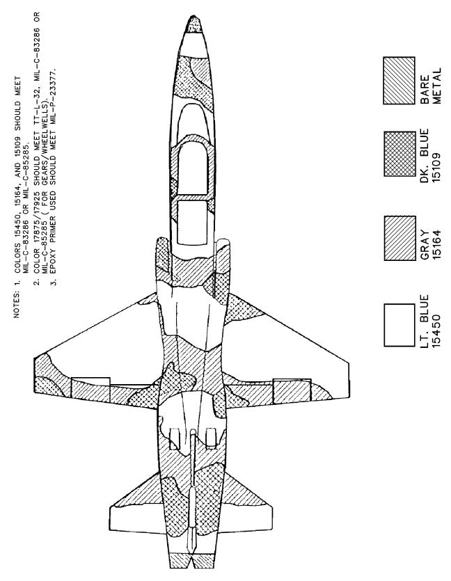
Figure D-29. AT-38B Aircraft Camouflage Pattern (Sheet 2 of 3)
