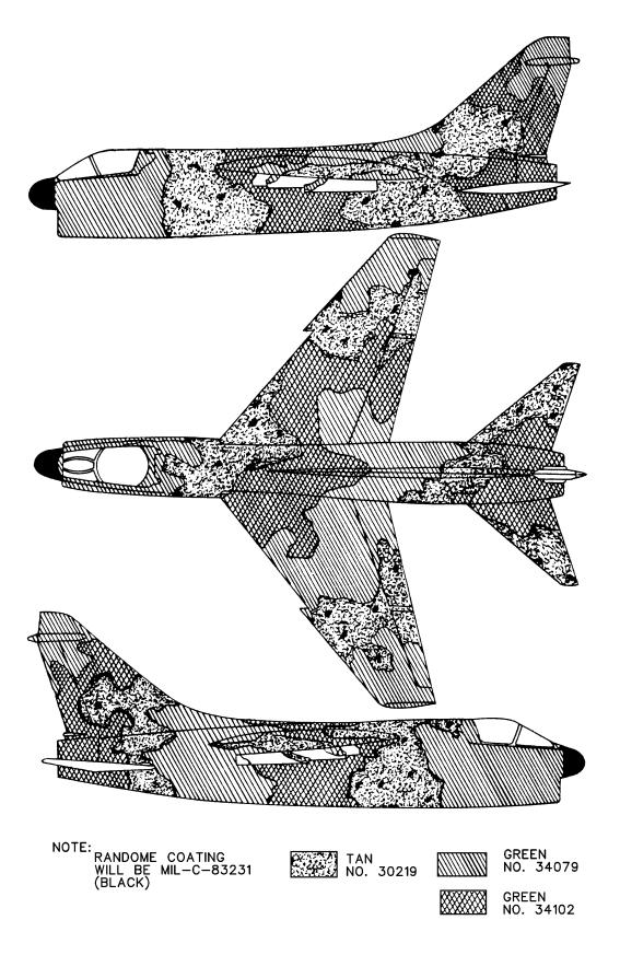
Figure D-1. A-7 Aircraft Camouflage Pattern (Sheet 1 of 2)
