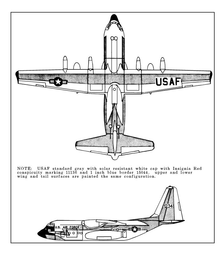
Figure C-2. RC-130 Aircraft Conspicuity Marking
