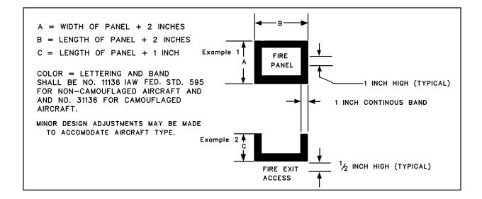
Figure E-4. Markings For Fire Access Panel
