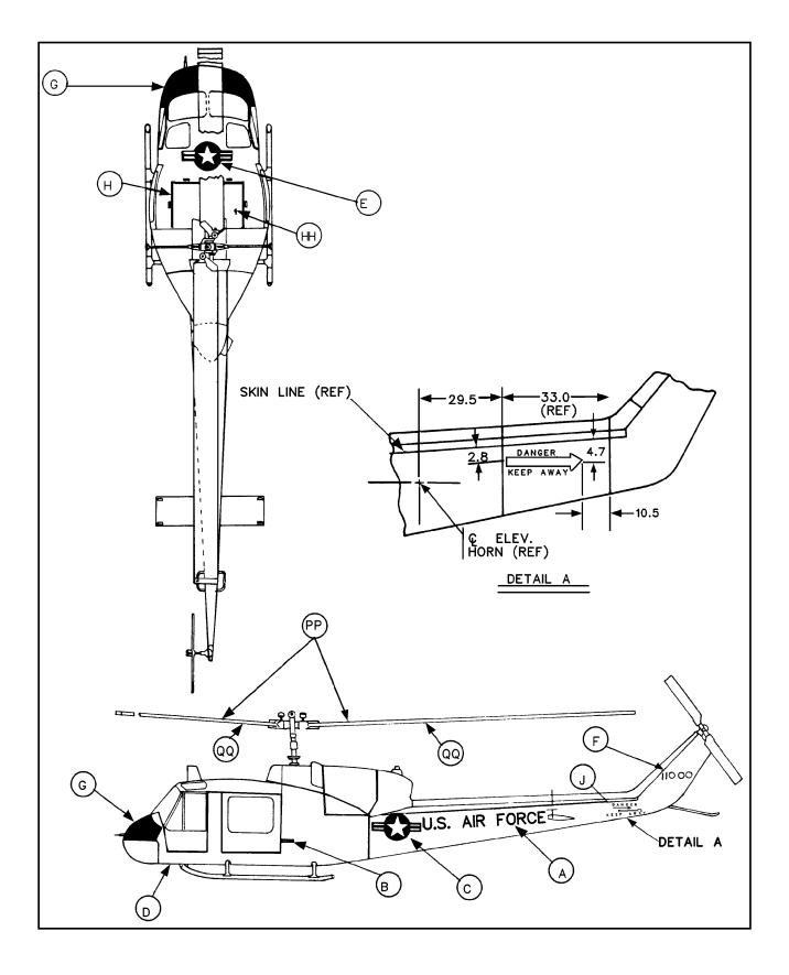
Figure B-10. H-1 Aircraft Marking Specification
