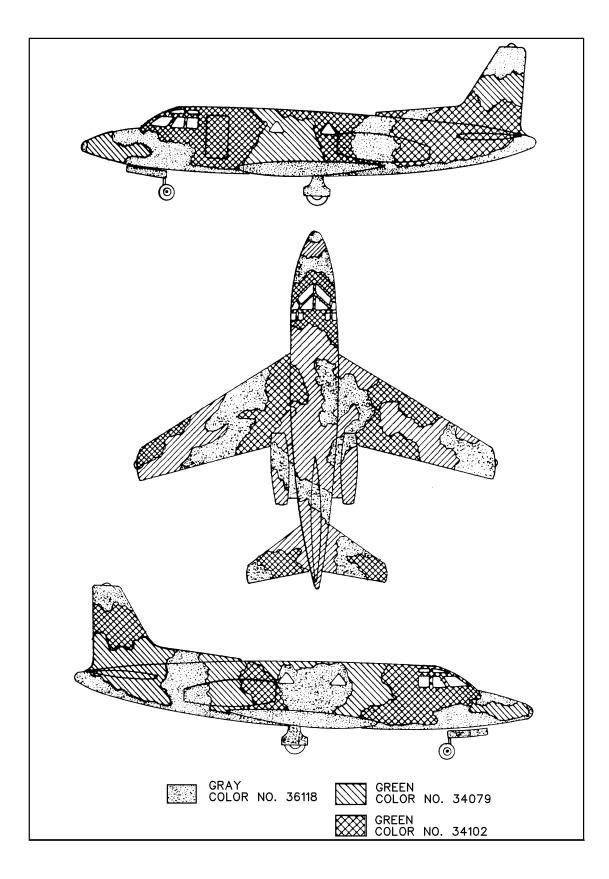
Figure D-30. T-39 Aircraft Camouflage Pattern
