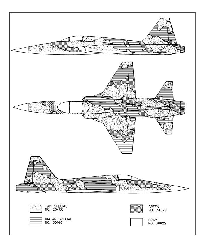
Figure D-14. F-5 Aircraft Camouflage Pattern For Asia Minor
