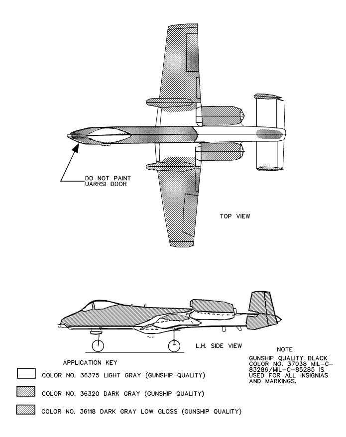
Figure D-34. A-10 Aircraft Camouflage Pattern for High and Low Reflectance Gray (Sheet 2 of 2)
