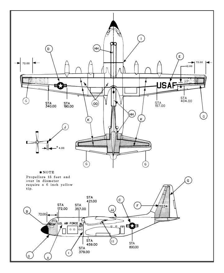
Figure B-5. C-130 Aircraft Marking Specification
