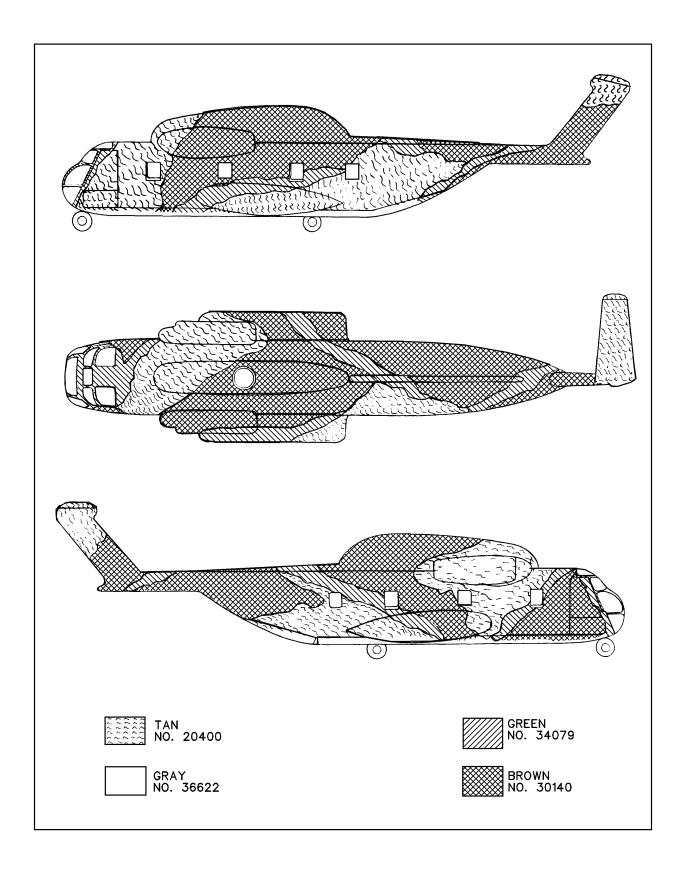
Figure D-26. HH-53B Helicopter Camouflage Pattern
