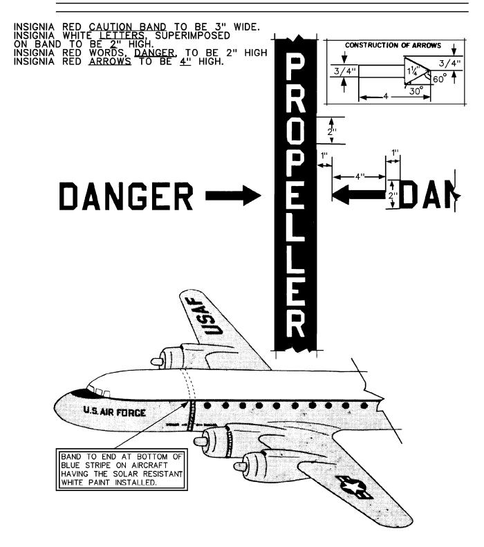
Figure E-10. Propeller Warning Stripes and Signs
