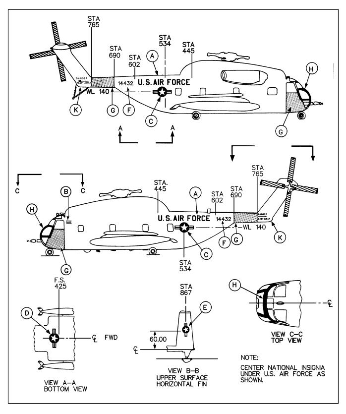
Figure B-13. H-53 Aircraft Marking Specification
