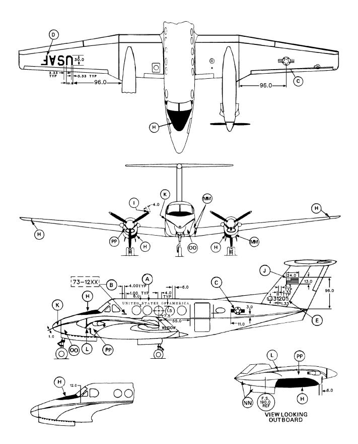
Figure B-4. C-12 Aircraft Marking Specifications
