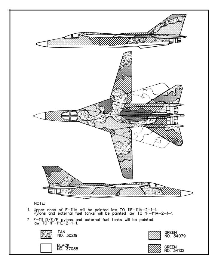
Figure D-15. F-111 A/D/E/F Aircraft Camouflage Pattern
