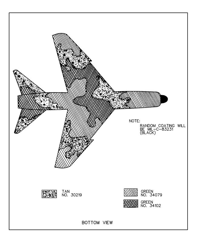
Figure D-1. A-7 Aircraft Camouflage Pattern (Sheet 2 of 2)
