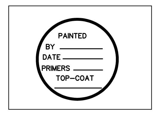
Figure A-5. Typical Marking For Paint Facility/Finish Identification Block
