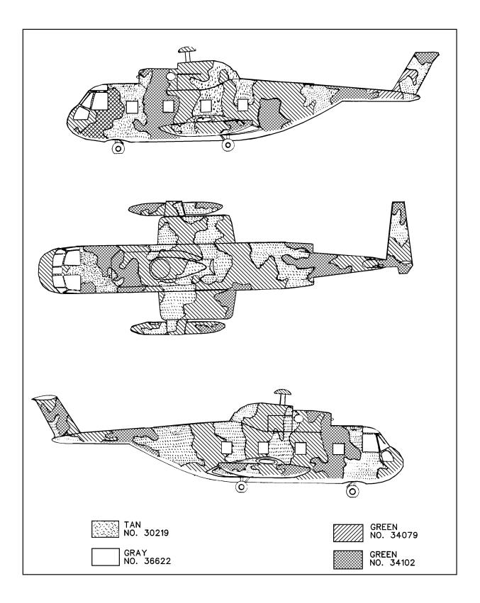
Figure D-21. H-3 Aircraft Camouflage Pattern
