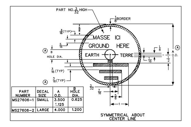
Figure E-3. Decalcomania - Ground Here, International Symbol
