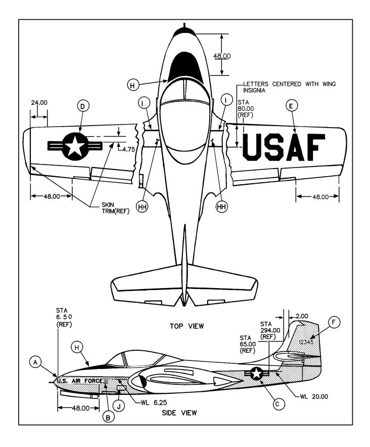
Figure B-17. T-37 Aircraft Marking Specification
