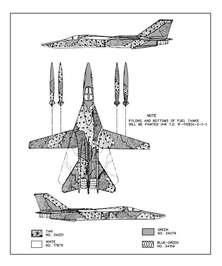
Figure D-16. FB-111A Aircraft Camouflage Pattern
