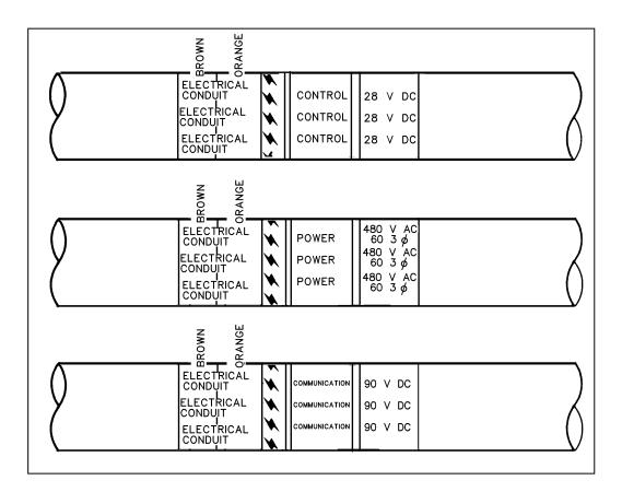
Figure F-5. Examples of Electrical Identification
