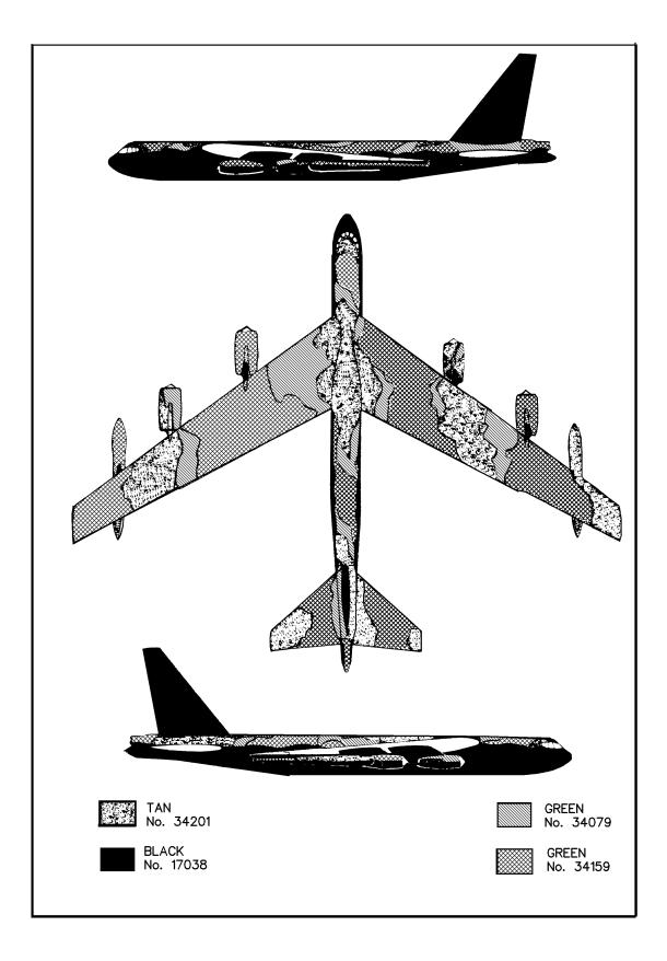
Figure D-4. B-52 Aircraft SEA Camouflage Pattern
