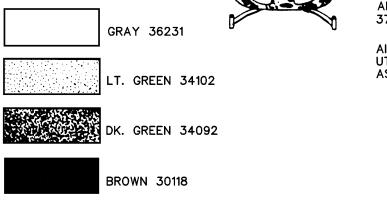
PAINT ALL PAINTED, NON-BLACK MAIN ROTORHEAD COMPONENTS AND TAIL ROTOR GEARBOX BLACK 37038.
