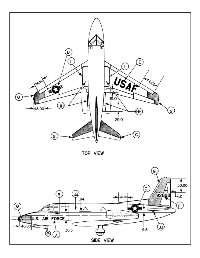
Figure B-19. T-39 Aircraft Marking Specification
