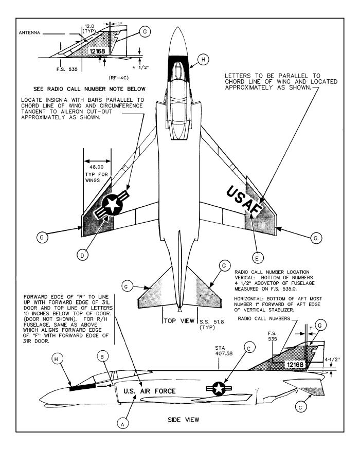
Figure B-8. F-4 Aircraft Marking Specification
