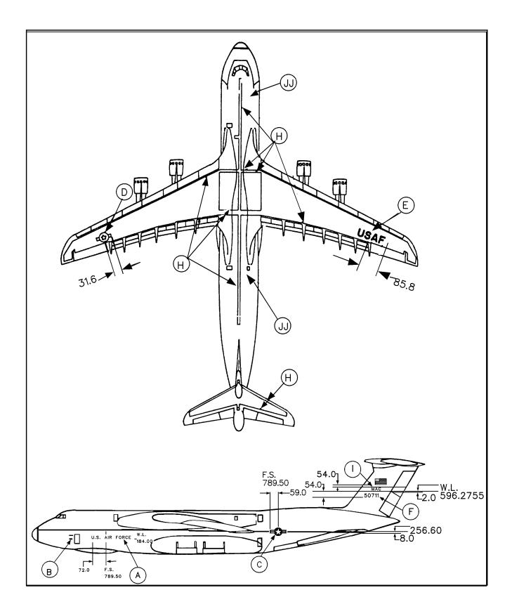
Figure B-2. C-5 Aircraft Marking Specification
