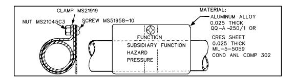
NOTES: 1. Tag sizes shall be compatible with the diameter of the tubing.
