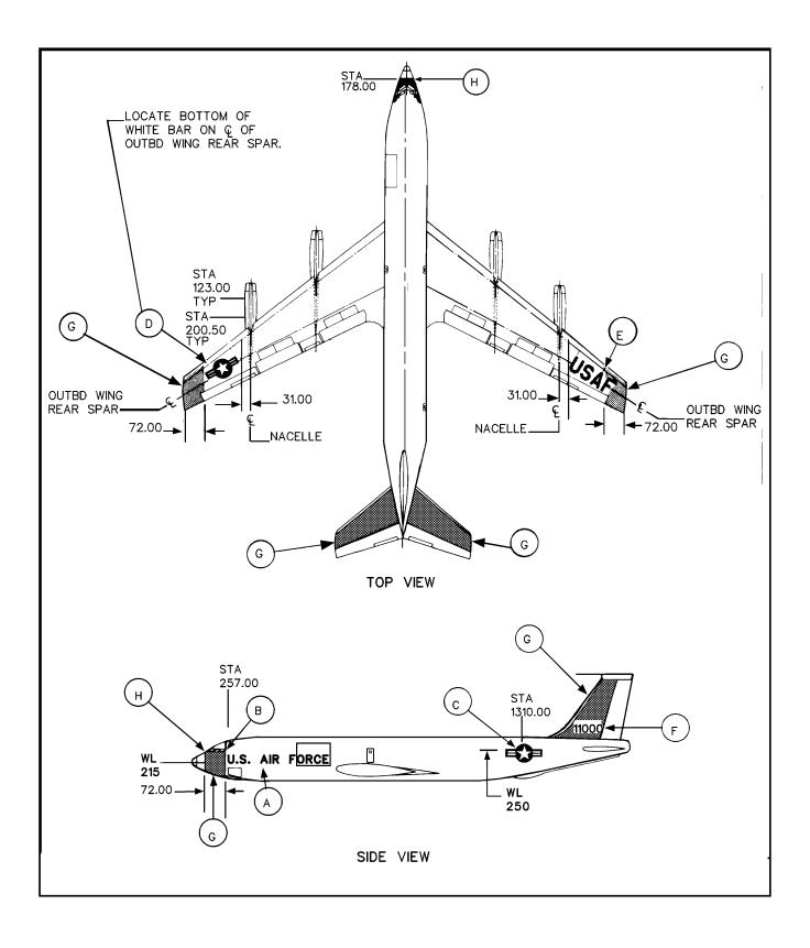
Figure B-6. C-135 Aircraft Marking Specification
