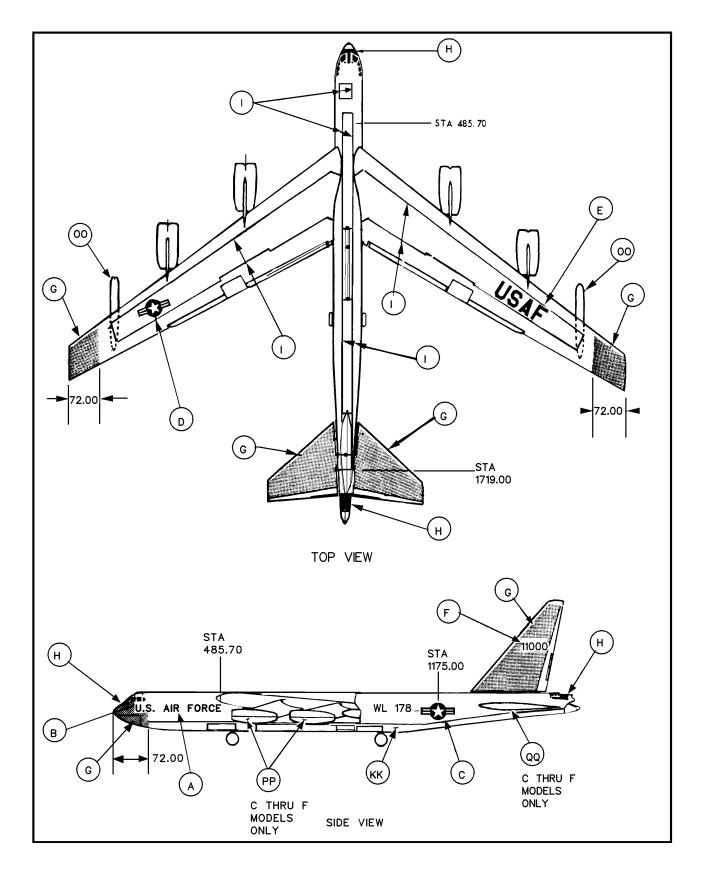
Figure B-1. B-52 Aircraft Marking Specification
