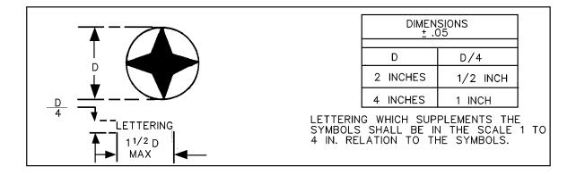
Figure E-1. Typical Symbol Dimensioning
