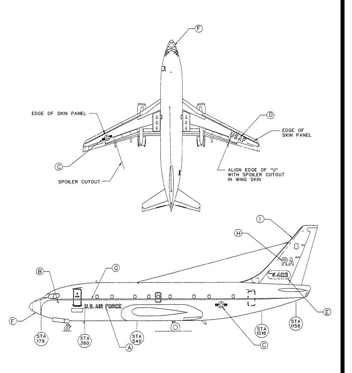
Figure B-21. T-43A Aircraft Marking Specification
