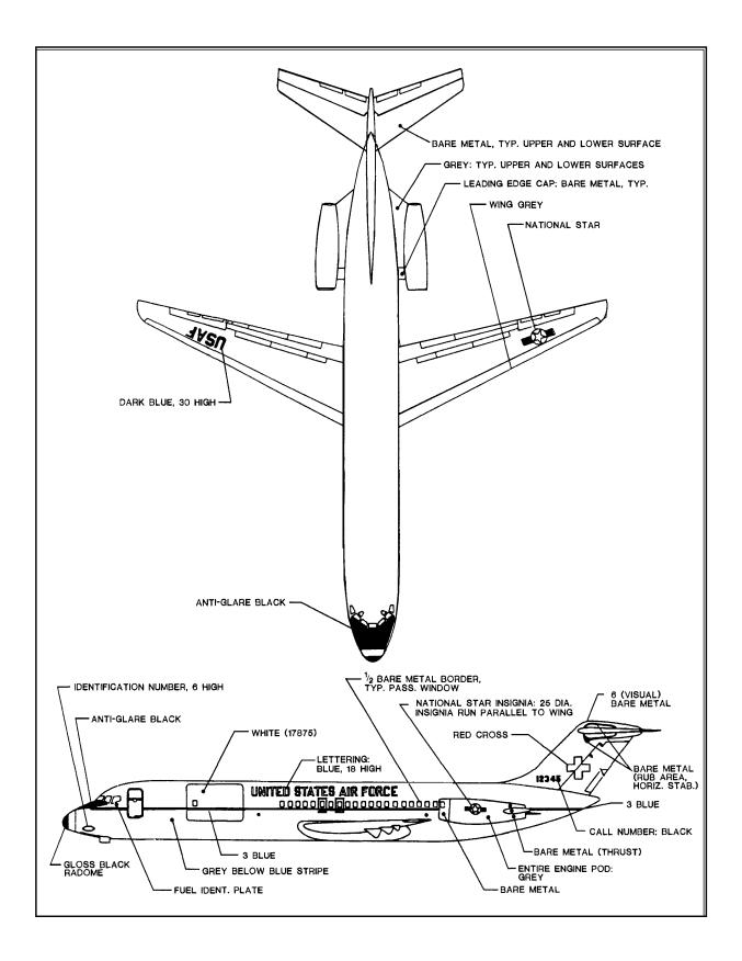
Figure B-3. C-9 Aircraft Marking Specifications
