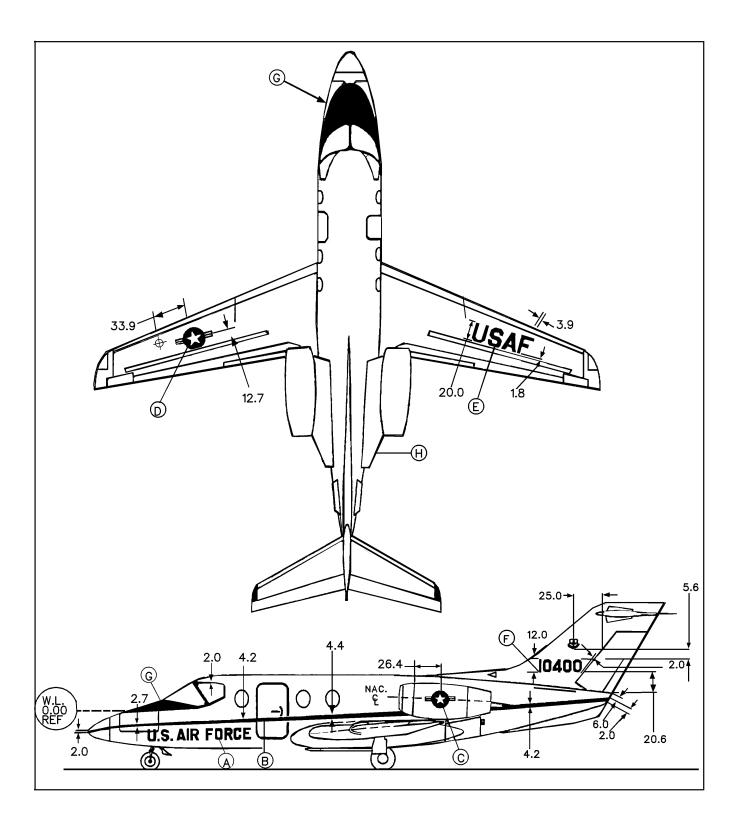
Figure B-15. T-1A Aircraft Marking Specification
