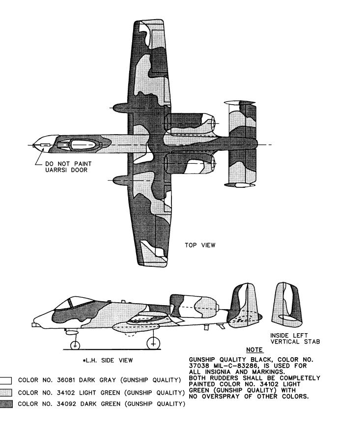
Figure D-33. A-10 Aircraft Camouflage Patten "European I" (Sheet 2 of 2)
