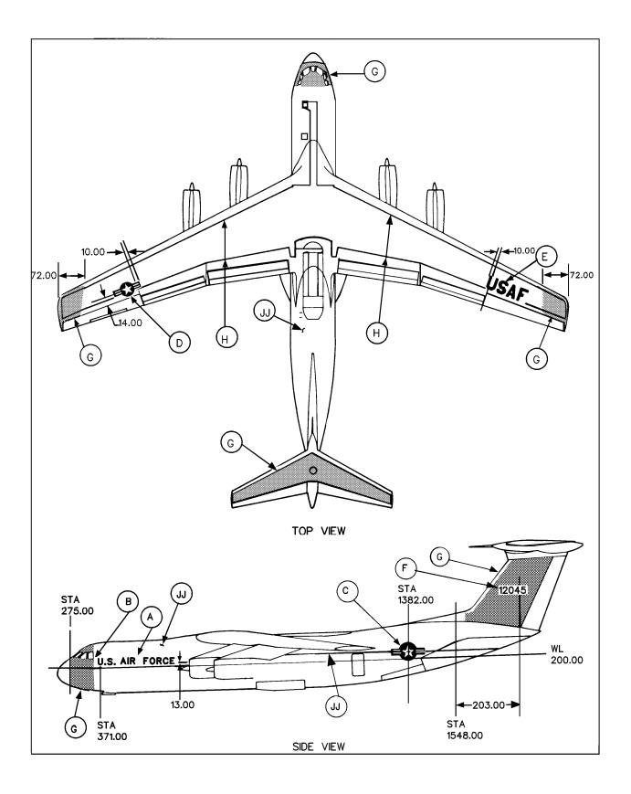
Figure B-7. C-141 Aircraft Marking Specification
