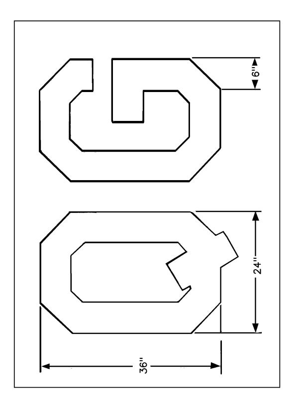
Figure D-37. Typical Distinctive Unit Aircraft Identification, 36" Letter Sizes
