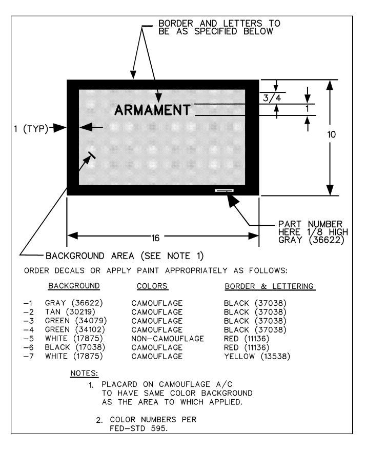
Figure E-8. Armament Placard Marking
