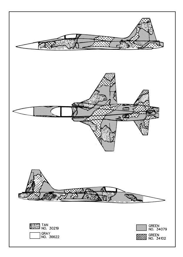
Figure D-13. F-5 Aircraft Camouflage Pattern
