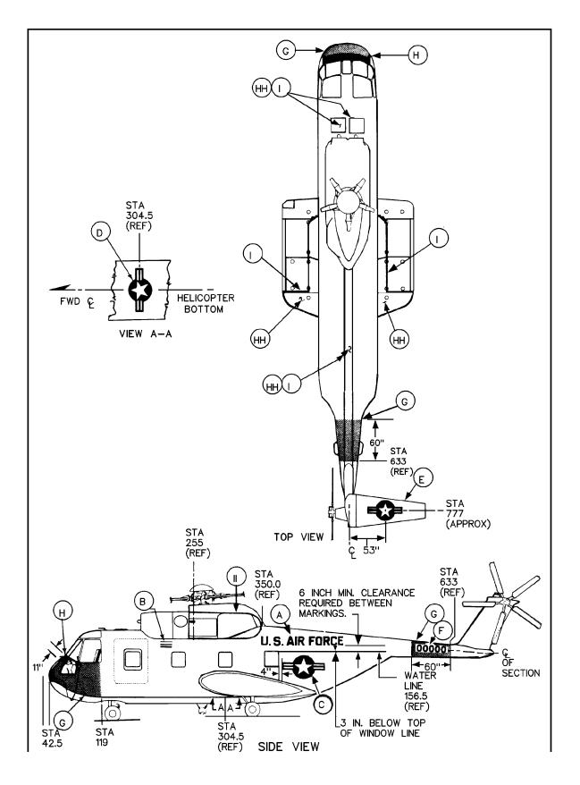
Figure B-11. H-3 Aircraft Marking Specification
