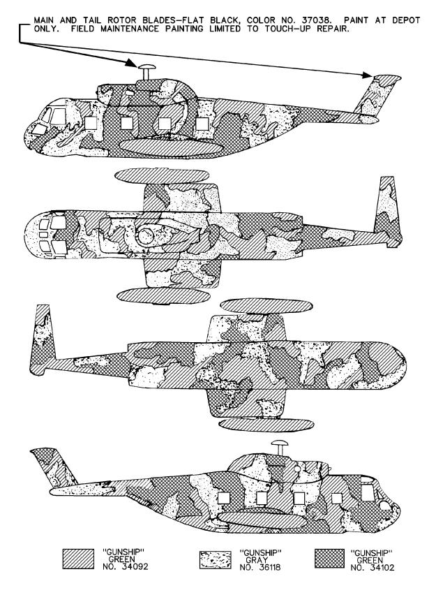
Figure D-23. CH-3 Aircraft European I Camouflage Pattern
