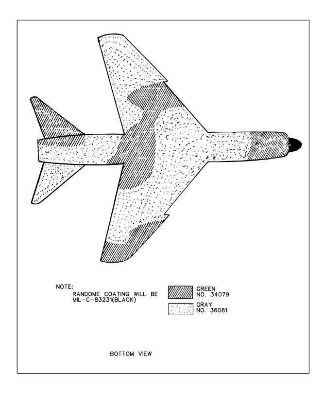
Figure D-2. ANG A-7 Aircraft Camouflage Pattern (Sheet 2 of 2)
