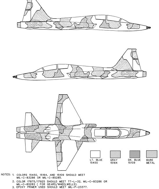
Figure D-29. AT-38B Aircraft Camouflage Pattern (Sheet 1 of 3)
