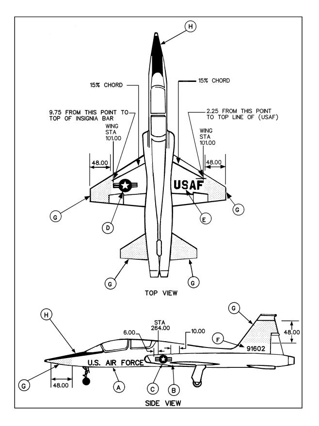
Figure B-18. T-38 Aircraft Marking Specification
