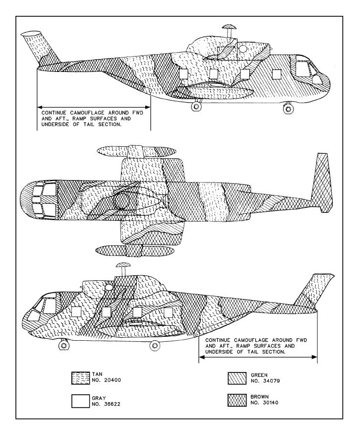
Figure D-22. CH-3 Aircraft Camouflage Pattern
