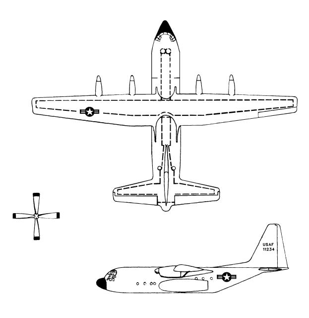
NOTE: ALL EXTERIOR FINISH AND MARKINGS SHALL CONFORM TO AF DRAWING 7434744, USING MIL-C-83286 "GUNSHIP" POLYURETHANE PAINT, COLOR CODE 36118.
