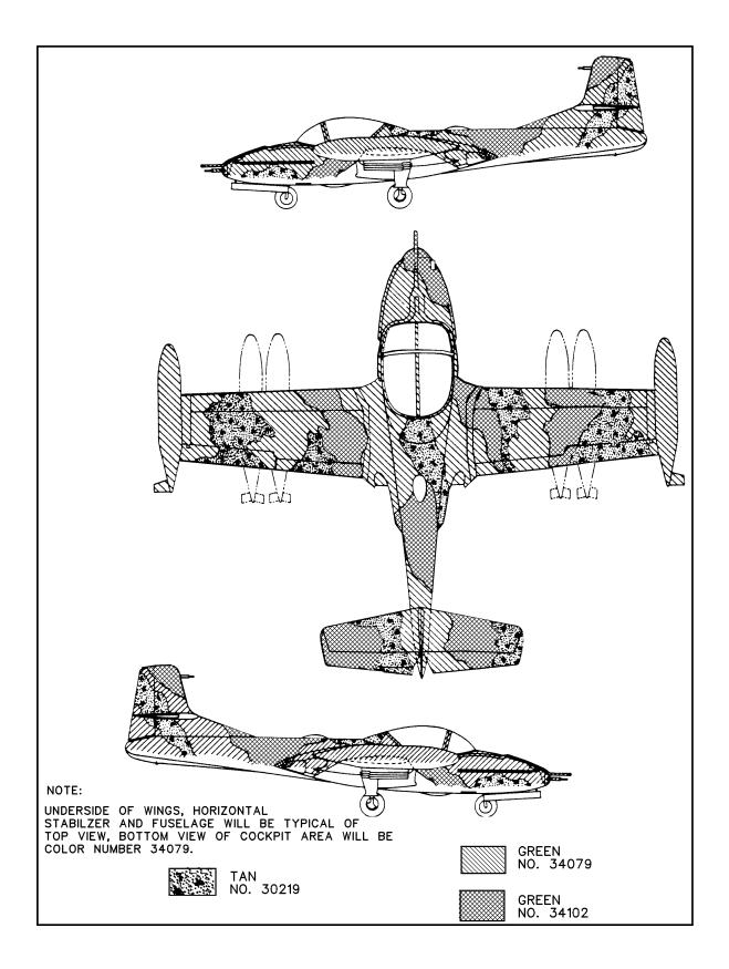
Figure D-28. A-37/OA-37 Aircraft Standard Camouflage Pattern
