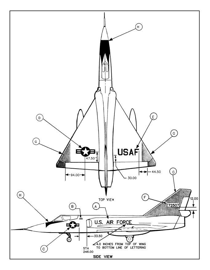
Figure B-9. F-106 Aircraft Marking Specification
