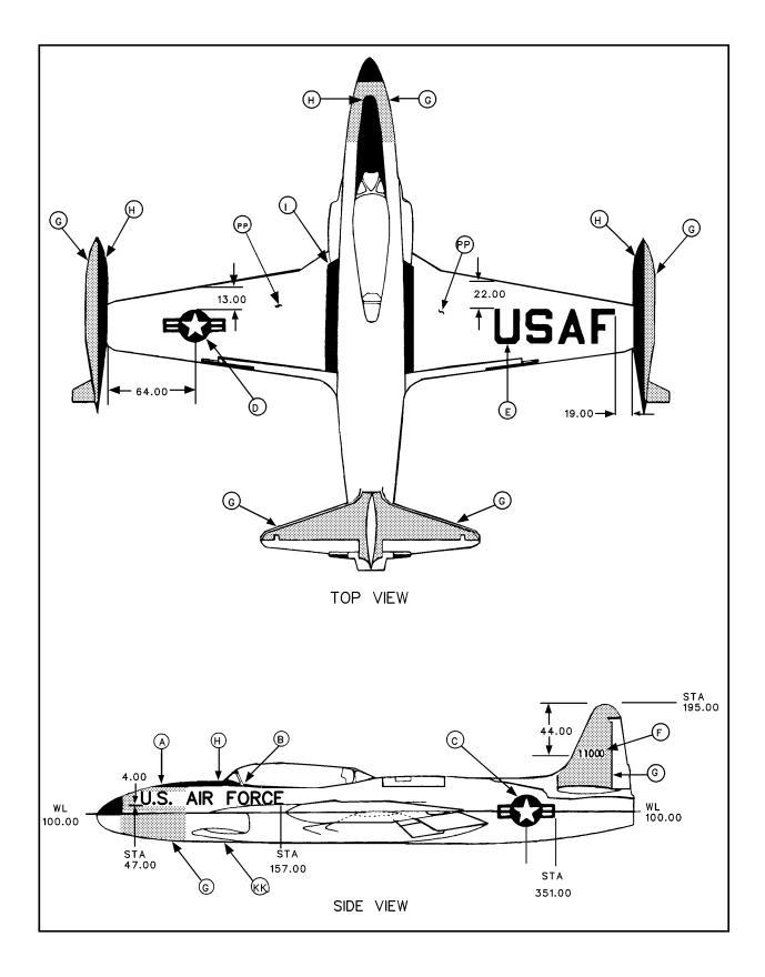
Figure B-16. T-33 Aircraft Marking Specification
