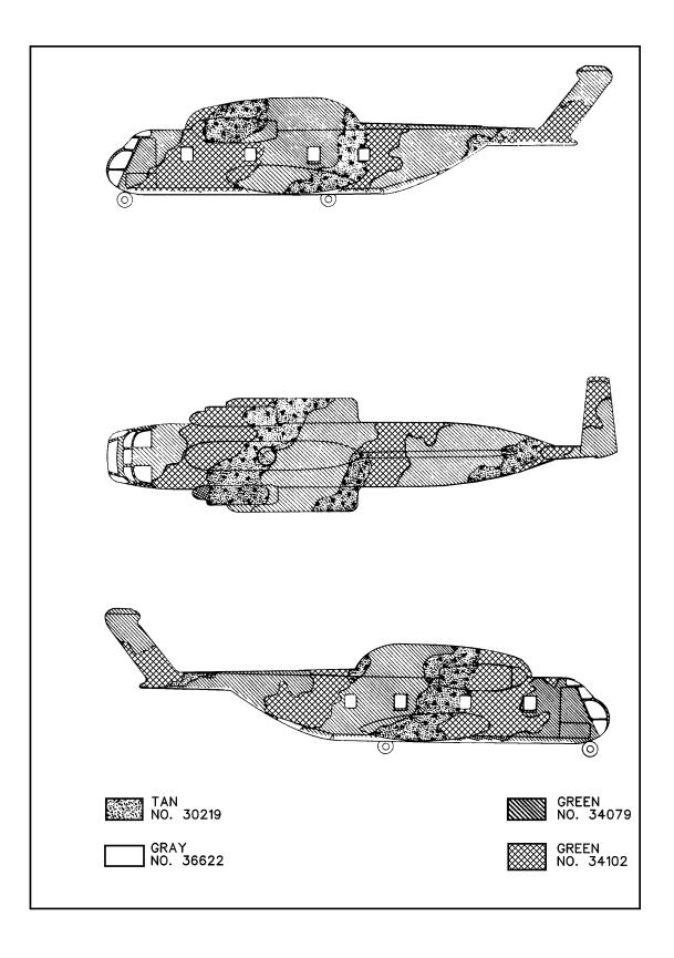
Figure D-24. H-53 Aircraft Standard Camouflage Pattern
