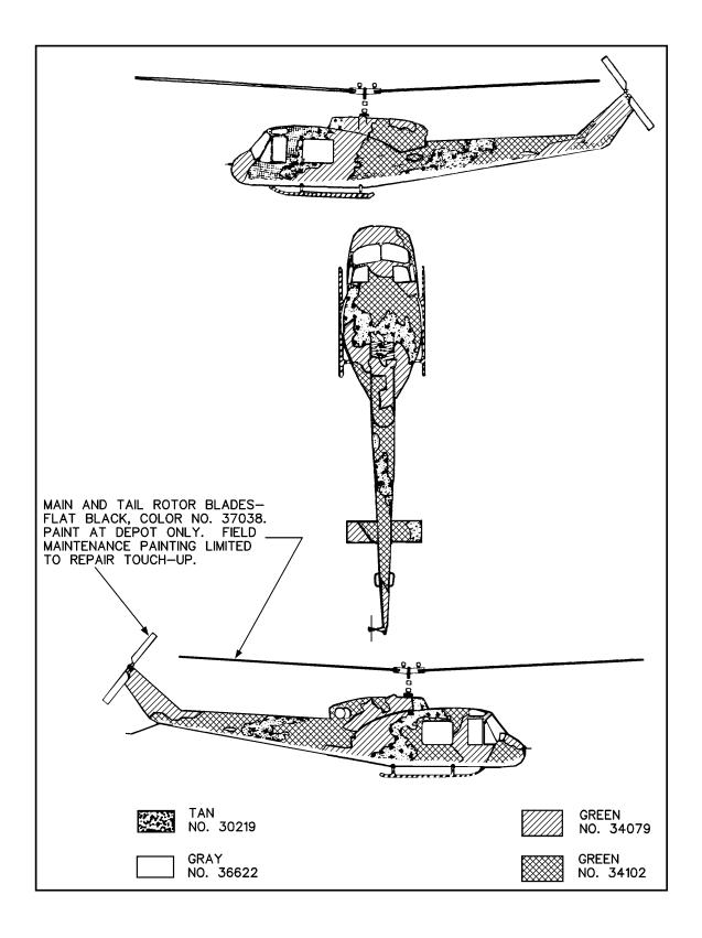
Figure D-17. H-1F/D/N/H Aircraft Standard Camouflage Pattern
